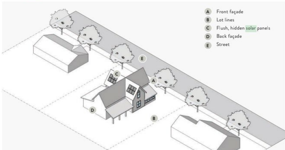
Fig 4.2 Solar Panels Placement
