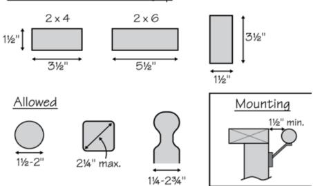
Handrails must be graspable and have a perimeter dimension of at least 4" and not greater than 6%." (A 2 x 4 is not allowed: 10" perimeter.)
