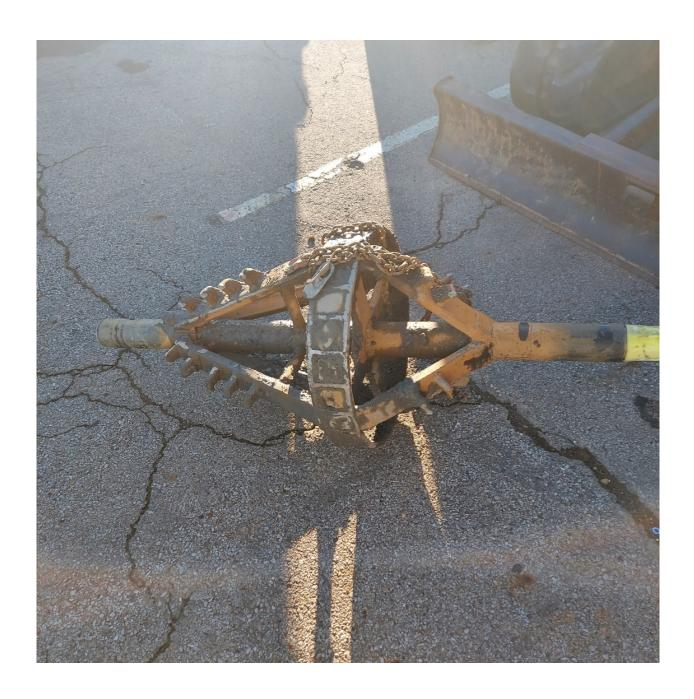
Horizontal Directional Drilling - Drill Head For 18-Inch Bore
